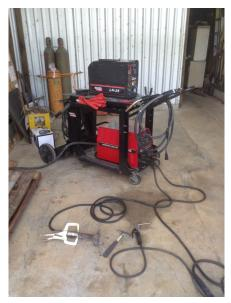
Our new Perkins 10KW power plant (left) powers our newly overhauled Lincoln Electric welder (right) in the hangar as well as powering the entire mission base and both wells. The generator was shipped in two pieces to allow loading into our MAG Cessna 206 aircraft. [More pictures on page 2.]
